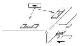
d) If anchor bolts have been pre-cast in the foundation slightly tighten the anchor bolts. Otherwise let them hang in the foundation holes.
